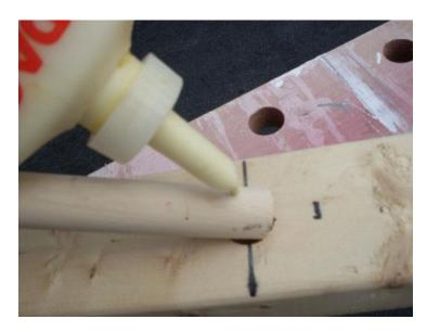
Drill a ½-inch hole through the center of 2x3s at each mark you made for the dowels. It is best to use a drill press to keep the holes are perpendicular to the 2×3. You can do it freehand, however take care to ensure the hole is drilled straight down through the 2×3. Using good quality carpenters wood glue, glue the dowel s into the holes, let the assembly dry overnight. When the glue has dried sand the structure removing any rough edges.
